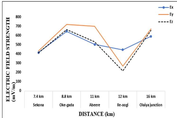
Figure 5: Electric Field strength against distance at secondary coverage region
