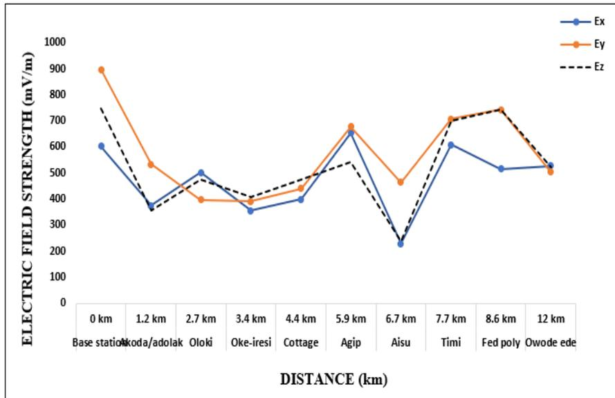
Figure 3: Electric Field strength against distance at primary coverage region
