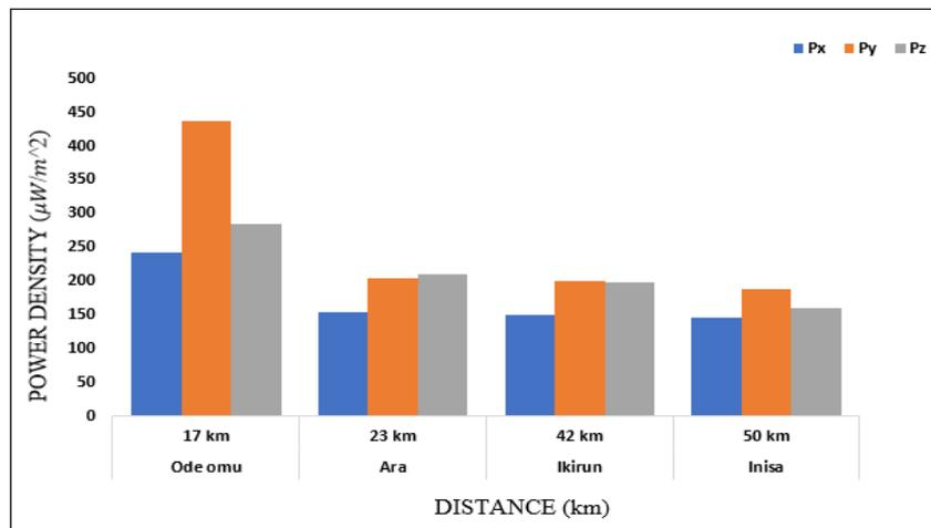
Figure 8: Power density against distance at fringe coverage region
