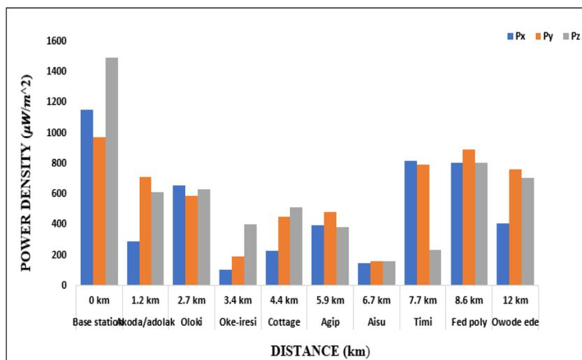
Figure 4: Power density against distance at primary coverage region
