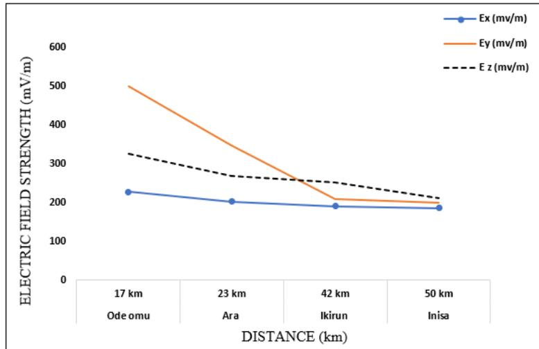
Figure 7: Electric Field strength against distance at fringe coverage region
