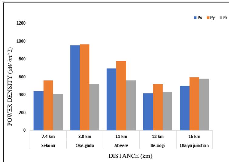
Figure 6: Power density against distance at secondary coverage region
